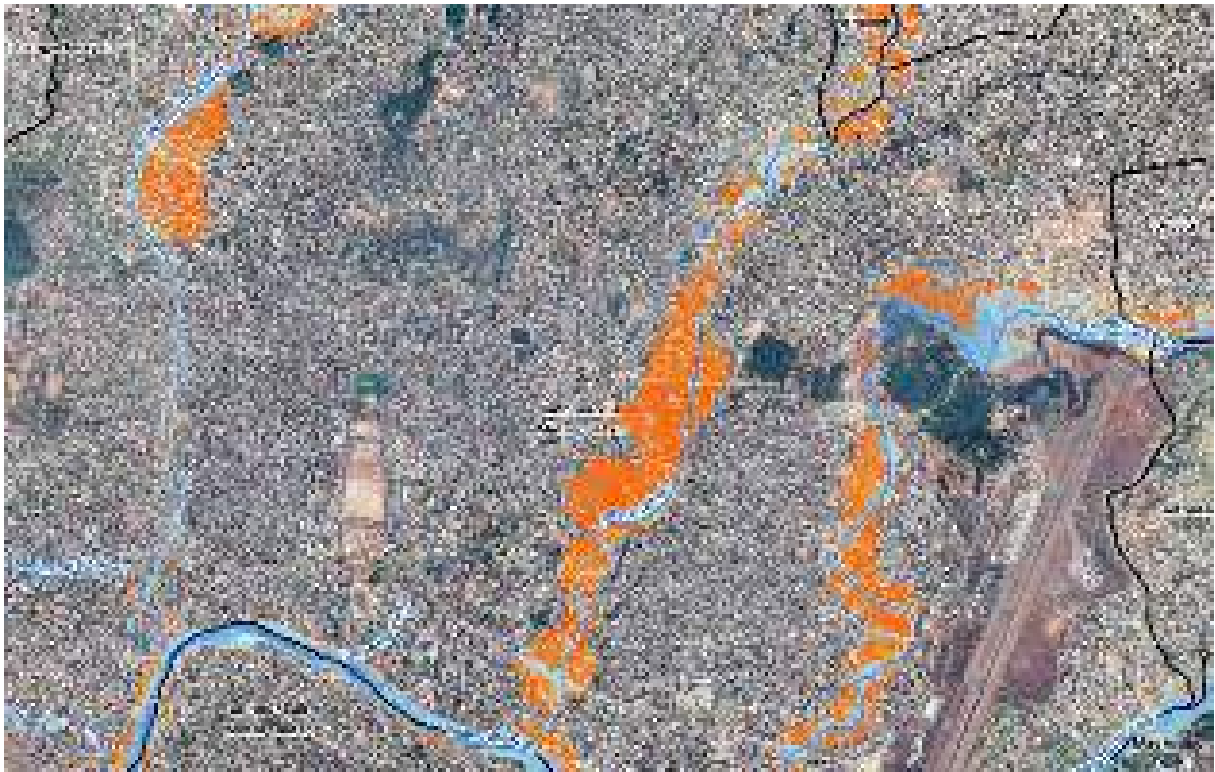
Figure 80 Inundated buildings by Dhobi Khola, Bagmati and Bishnumati Rivers for 100 years return period flood
